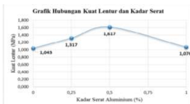
Figure 1.1 Graph of the relationship between flexural strength and fiber content (Source e-Jurnal MATRIX CIVIL ENGINEERING Vol. 2 No. 2/July 2014/109)
